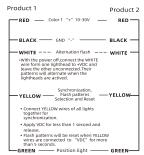
When the red wire and the green wire are connected together then warning light function will take precedence over the position light
